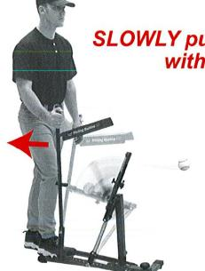
SLOWLY pull the RELEASE HANDLE with a smooth motion for the most accurate pitches.
