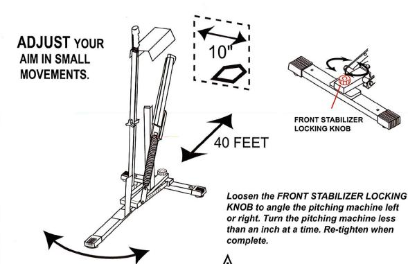
REMEMBER that turning the pitching machine 1/2" will move the pitch 10" at a distance of 40 feet.
